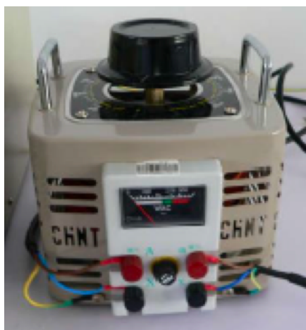
Photo of Voltage Regulator
