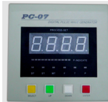
Photo of Digital Pulse Modulator Panel
