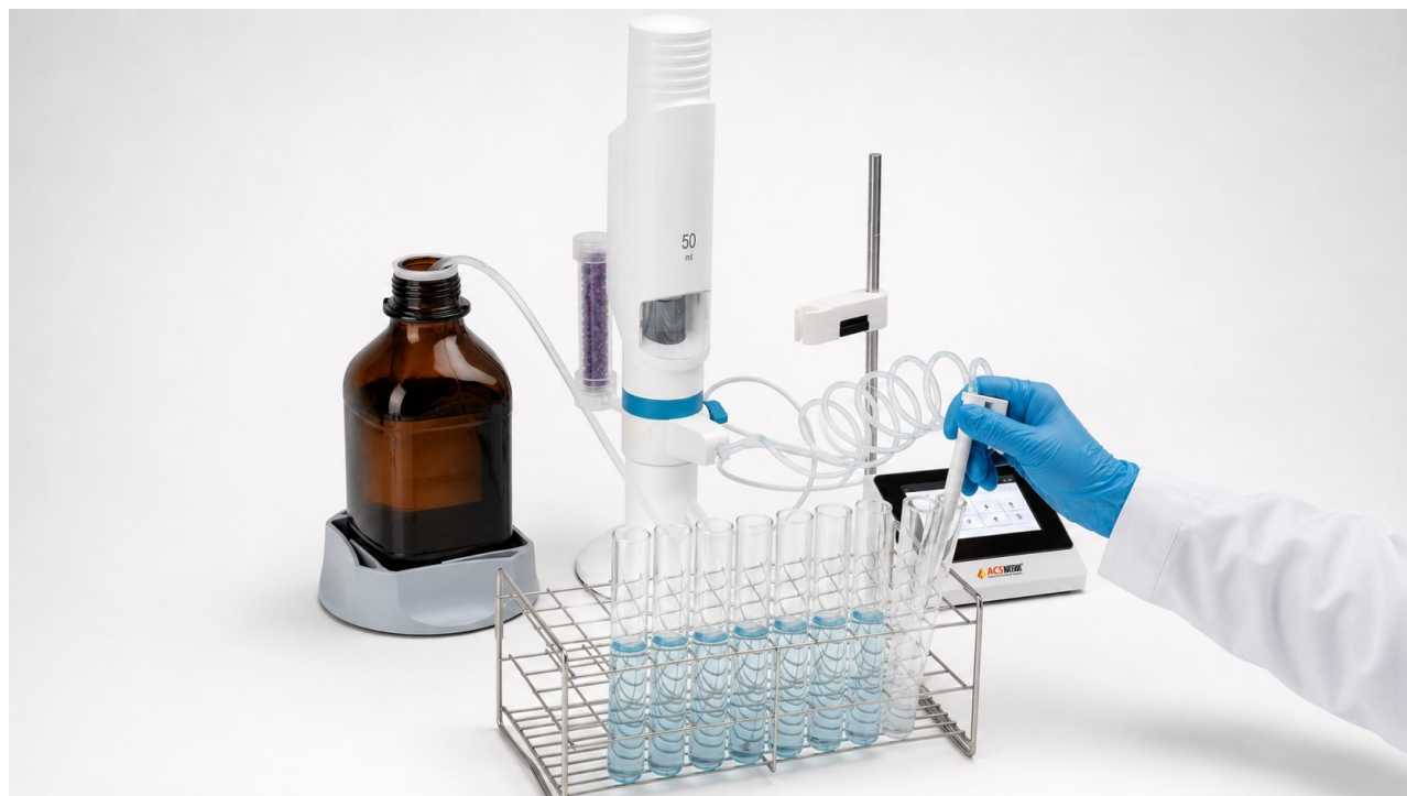
ACS Material ALab™ dFlow-Pro Electronic Bottle-Top Dispenser
