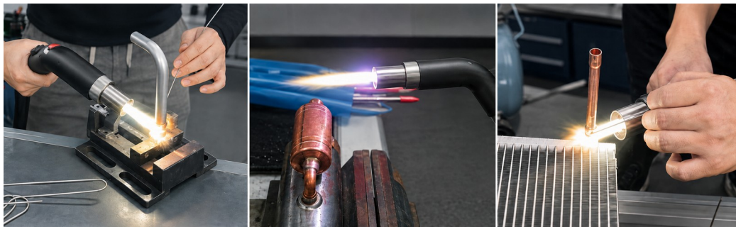
PlasmaNova™ plasma torch in a materials welding application.
